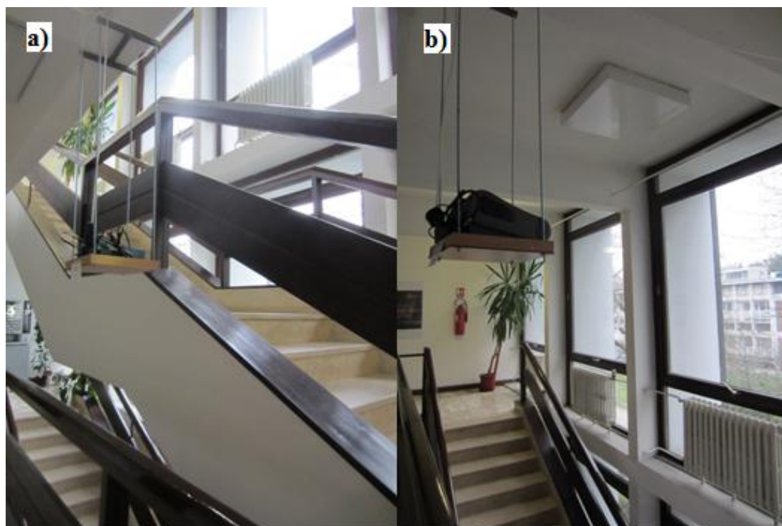
Fig. 3: Location of DUSTTRAK™ monitors a) ground floor, b) first floor. Both monitors were suspended so the inlet was at average breathing height of 1.7m.
