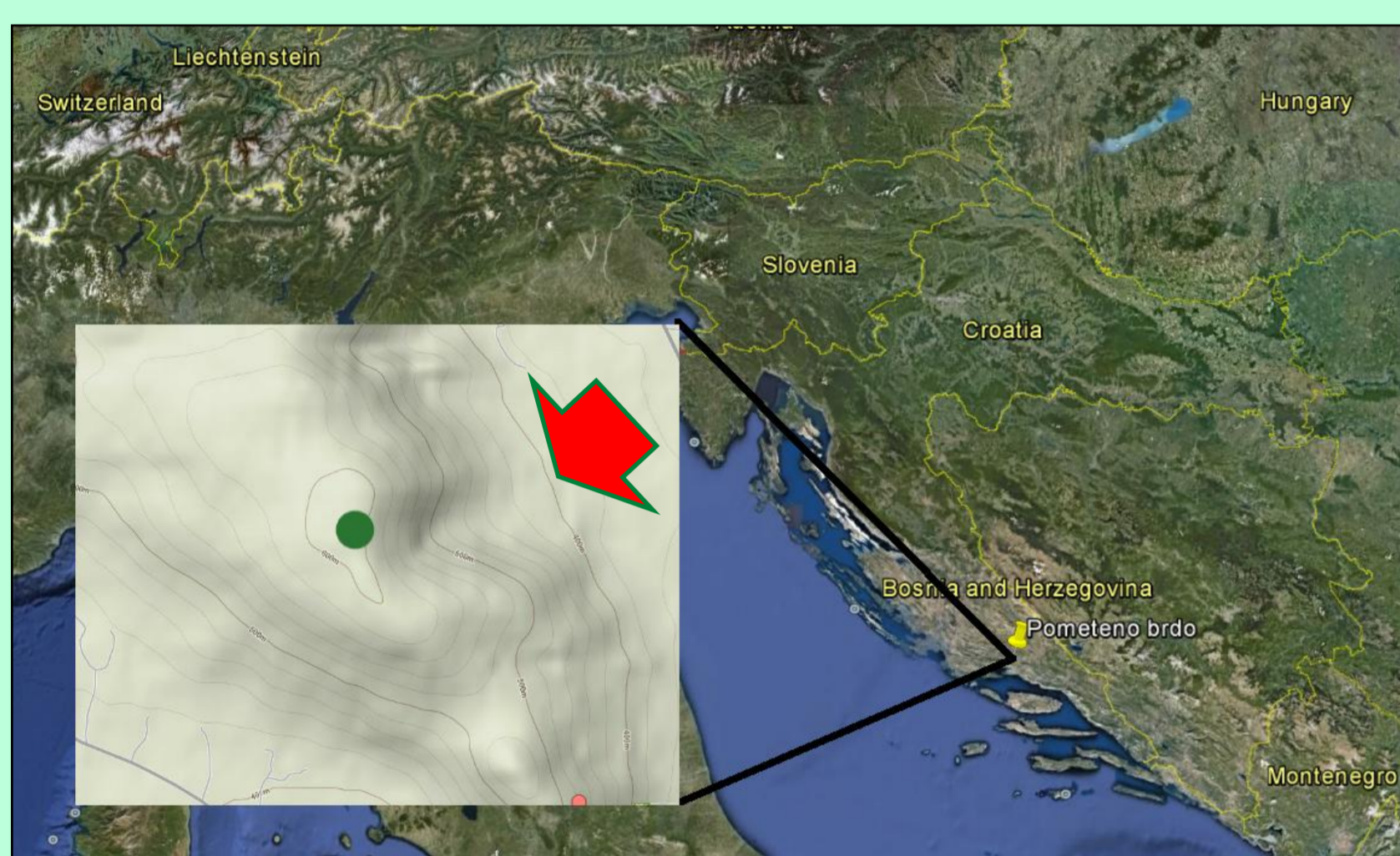
Fig.1. Site of Pometeno brdo: zoomed picture shows terrain and orientation of the hill relative to the mean bora direction (red arrow). Green circle denotes the position of the tower with anemometers.
