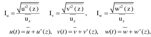
*u*, *v*, *w* time averaged mean wind velocities in the *x*-, *y*- and *z*- direction u', v', w' the respective fluctuating wind velocity components
