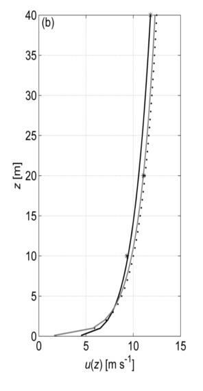
Star – measured median value Black solid line – power-law Black dotted line – logarithmic-law Grey line – direct adjustment of the log-law For entire 62 hours of measurement one mean velocity
